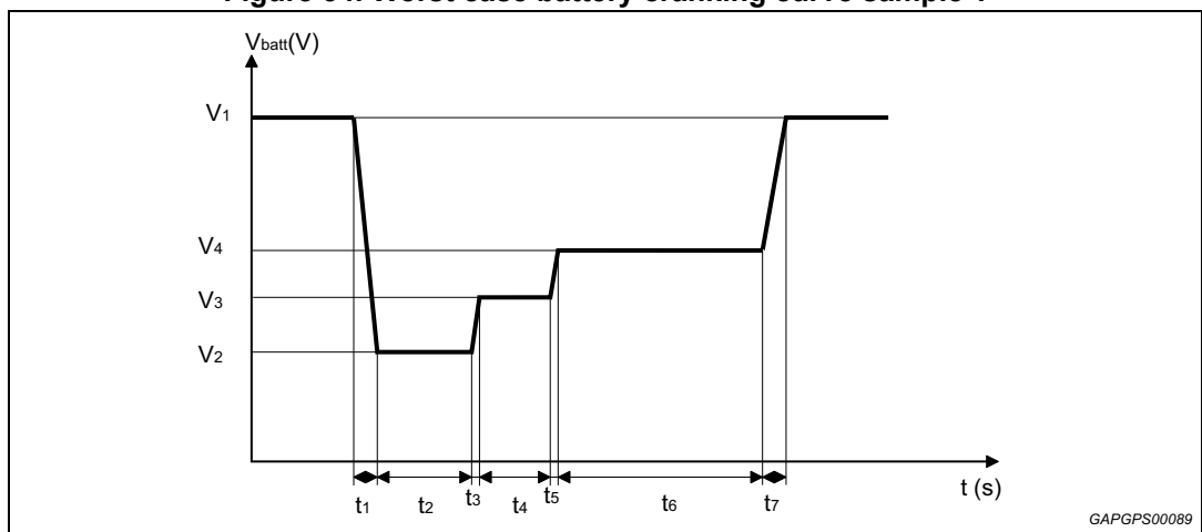
Figure 34. Worst case battery cranking curve sample 1
